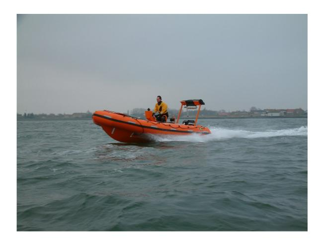
The RIBO600 is a larger boat, giving improved comfort, compared with the standard tiller steering rescue boats, like the RIBO450. It comes with a steering console/jockey seat and 2 additional jockey seats. This boat has been approved according to the latest SOLAS requirements for rescue boats, including IMO MSC.274(85) (weight definition 82.5 kg per person) and MSC/Circ. 1006 (improved fire retardancy).
