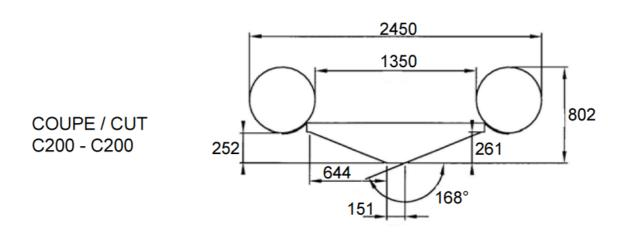
hull details, dimensions in mm
