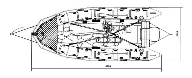
Overall dimensions (mm) with lifting sling, refer to page 5 and 6 for hull details dimensions and weight +/- 5%
