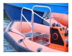
The WRH635 is self-bailing as the deck of the boat is above the water level, even while the boat is not running at speed. This is a unique system for this size of Fast Rescue Boats and increases its level of comfort.
