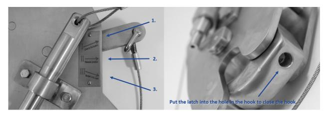
We recommend, to pull the handle and cord during lowering, just before the raft is waterborne. When waterborne, the hook will automatically open and the raft can be maneuvered away from the vessel. If a towing strain, or waves keep a load on the hook, the automatic function will not release the raft, then pull the handle/cord once more to release the hook.
